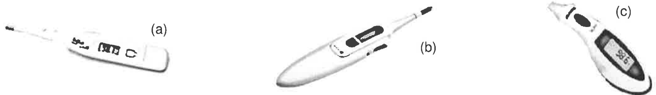
Picture 1 (a) Oral digital thermometer; (b) Rectal digital thermometer; (c) Digital ear thermometer.
